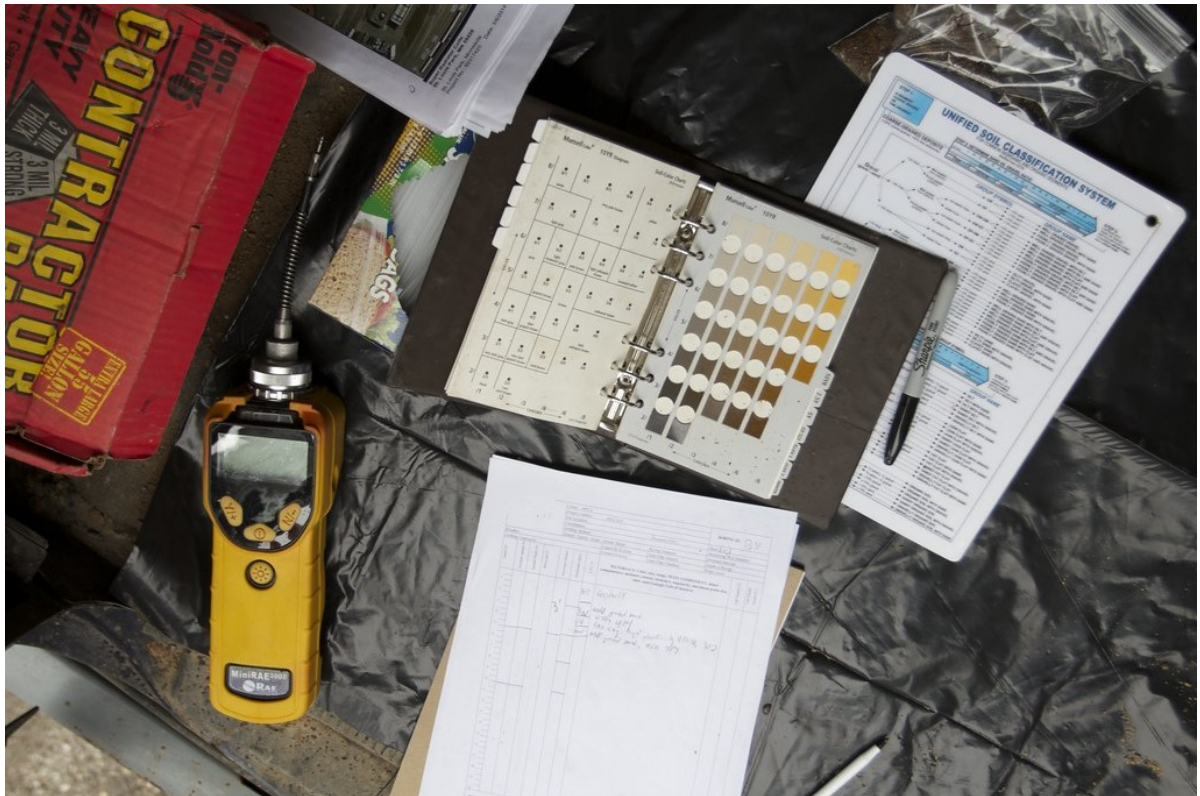
Figure 2. Soil color and classification charts used as references to complete field forms.
