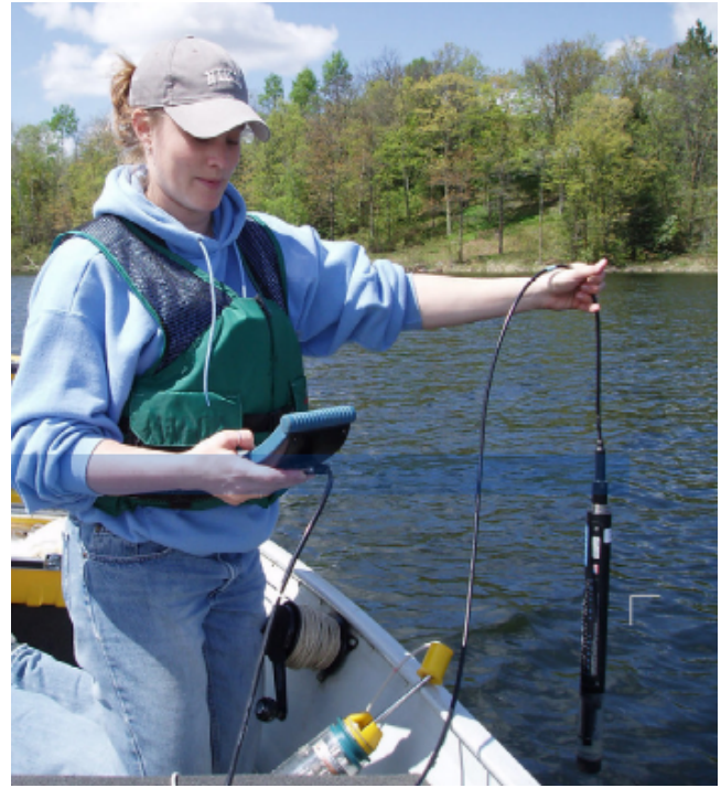
Figure 3. Field technician using low-volume point sensor.
